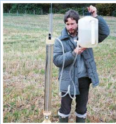
2) Install Permeameter and fill with water
