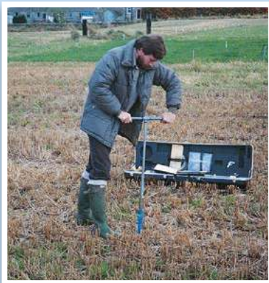
1) Auger and prepare hole
