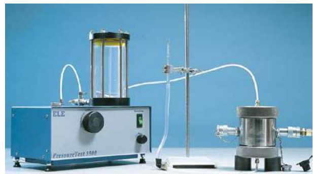
Permeability Test with Pressure Test 3500 Pressure System.
